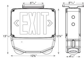
LETTER COLOR **HOUSING COLOR** MODEL No. of FACES **OPTIONS LLCWLEZXTEU** 1 Single Face R Red W White RC Remote Capacity CW Cold Weather Double Face G Green В Black SDT Self-Diagnostics CUSTOM **Custom Wording** G Gray (with white TP Tamper-Proof faceplate)
